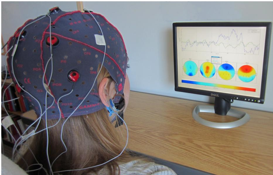
**Figure 1:** A participant wearing an eight-channel EEG cap while performing experiments in the Colorado State University BCI Laboratory. A small amount of electrically conductive gel is placed under each electrode in order to reduce the impedance between the sensors and the scalp.
